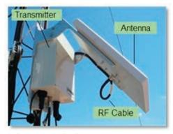
The Model 9502 includes 10 meters of RF cabling, granting the user freedom to position the antenna remotely and away from the transceiver in complex installations while securing the SIM card inside a premise or enclosure to better protect against unauthorized use, theft, and vandalism.
